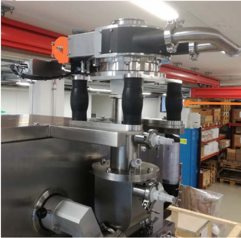
SBV valve powder inlet
