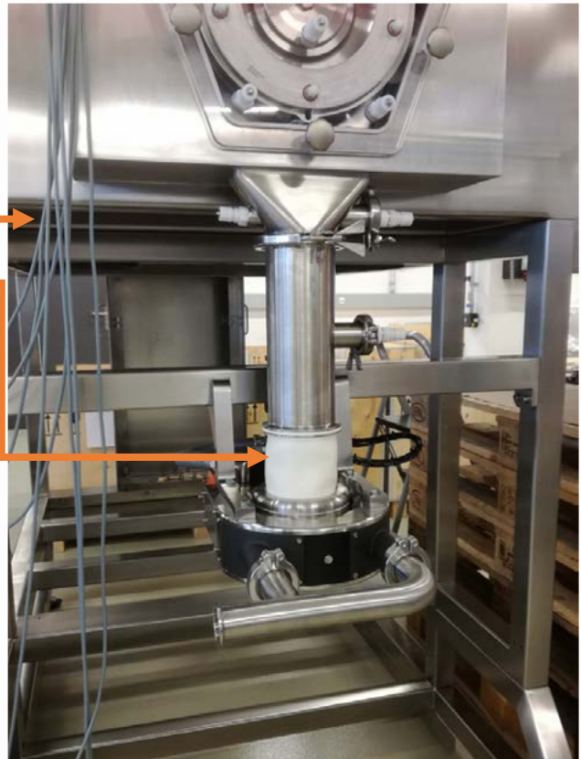
SBV valve granules outlet
