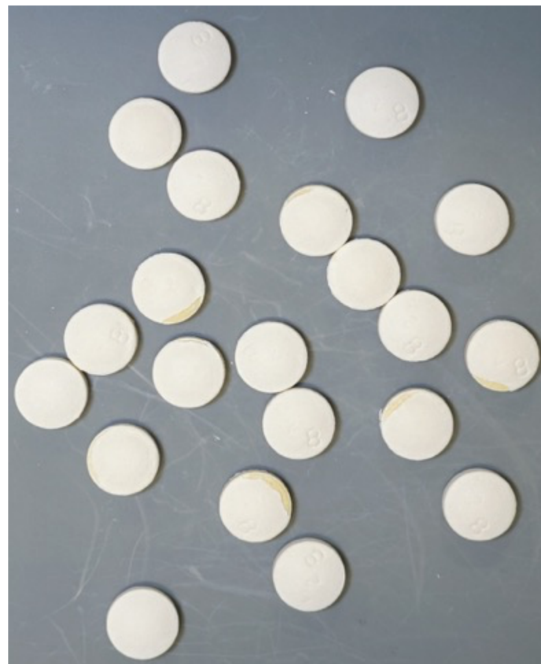
Figure 48: Appearance of tablets coated the TiO 2 -free COAT-010 (Rice Starch+D) versus TiO 2 -free COAT-027 (CaCO 3 +D)
