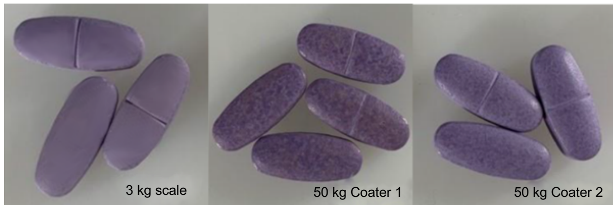
Figure 6: Evaluation of the visual appearance of a multivitamin tablet core coated with a purple TiO 2 free coating system at different scales and equipment type
